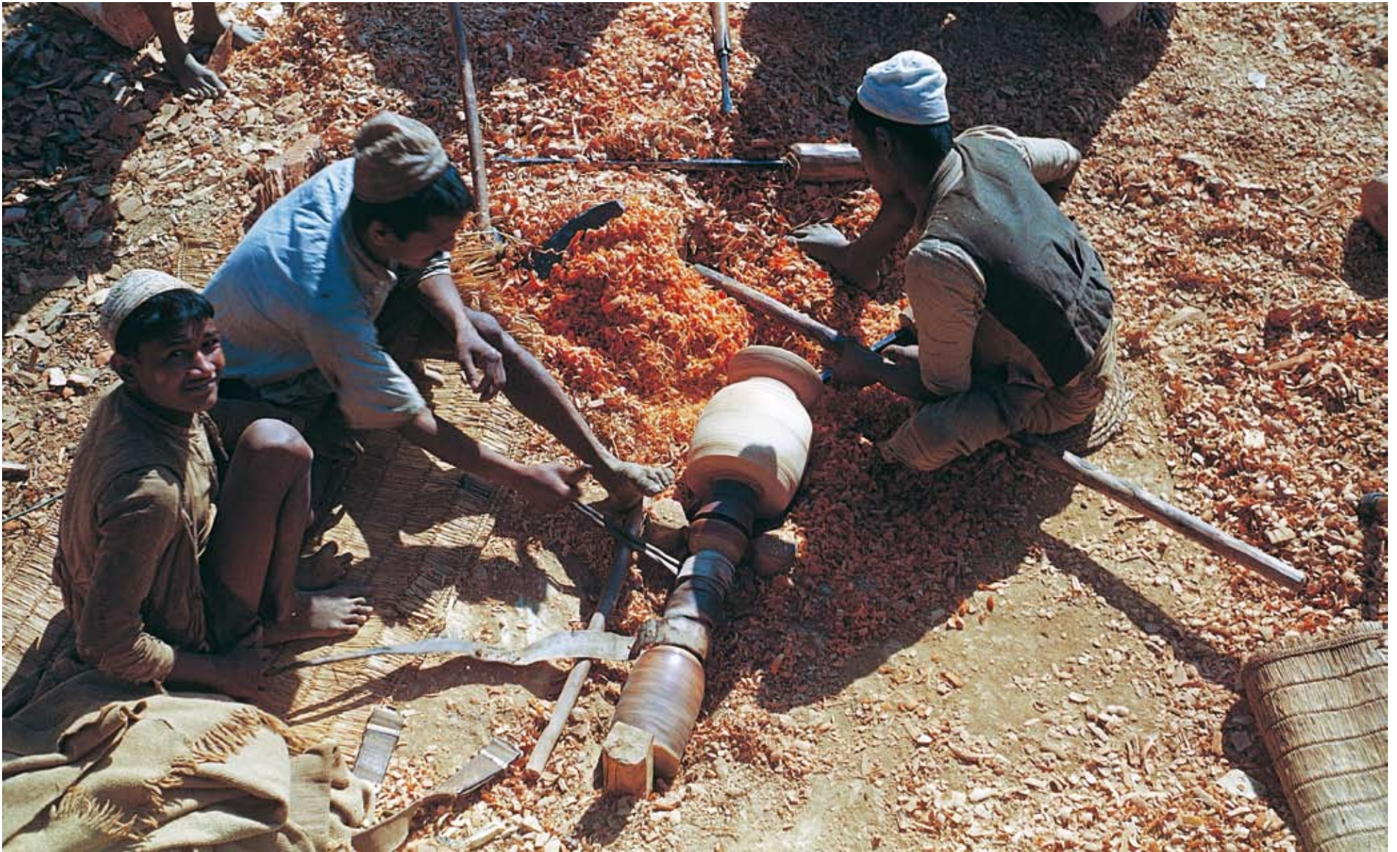
Making wooden vessels from heartwood is an age-old tradition. The axle is driven by hand straps but has now been largely replaced by electric motors.
