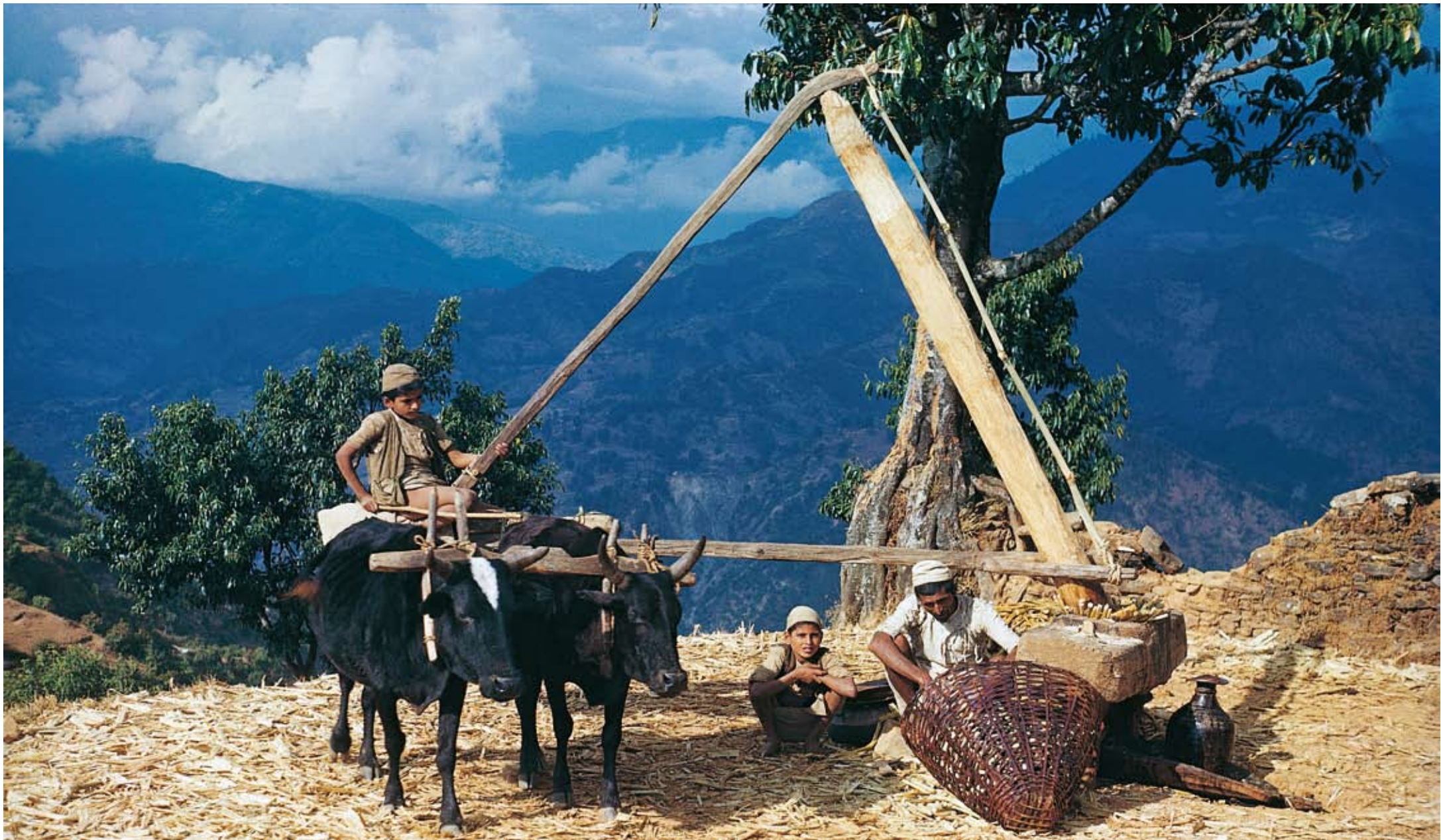
The machine to express oil from mustard seeds is run by bull power. Remote areas in Nepal still use this technique.
