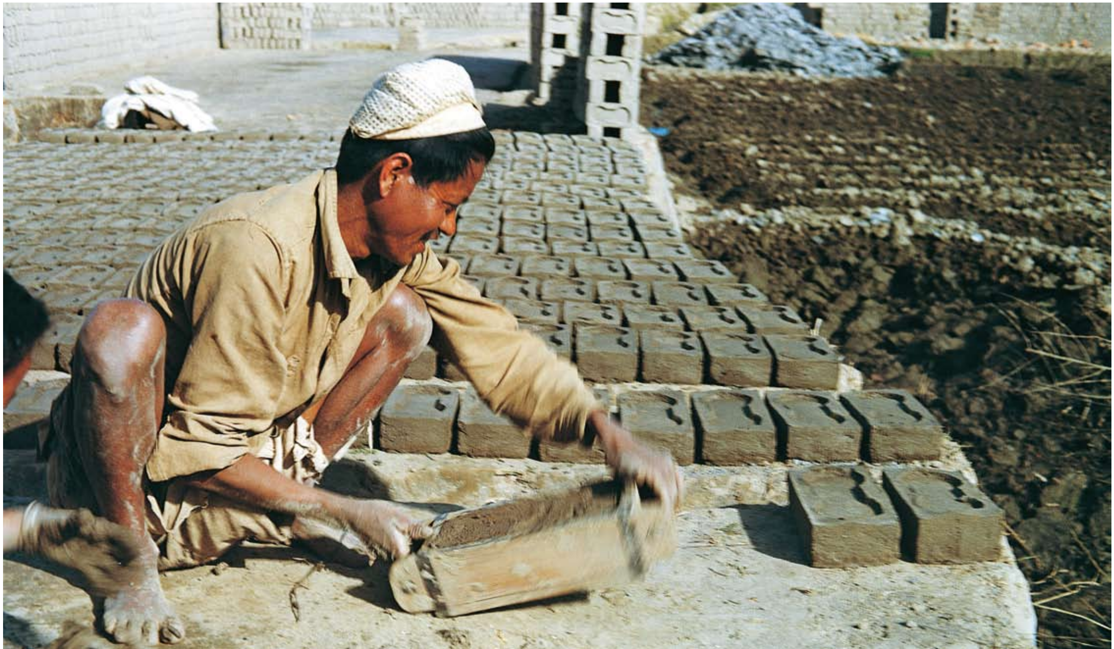
Mud bricks are sun baked before going into the kilns. The Kathmandu Valley was famous for its bricks and tiles and is now equally infamous for the pollution caused by brick kilns.
